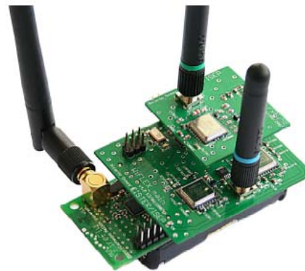
WiFLEX platform stacked on FireFly mote
