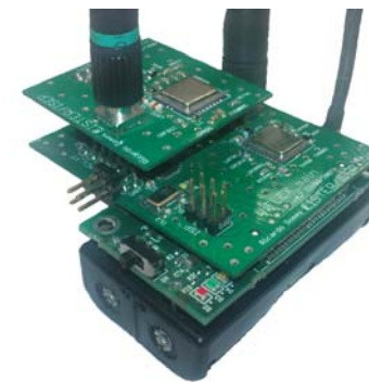
WiFLEX platform stacked on MICAz mote
