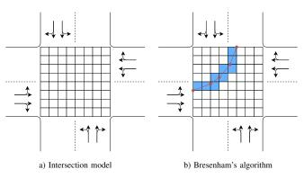
Fig. 1: Intersection modeled as a matrix of reservation tiles
