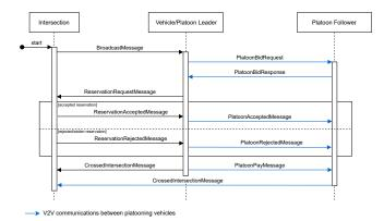
Fig. 2: V2X message flow of the intersection reservation mechanism
