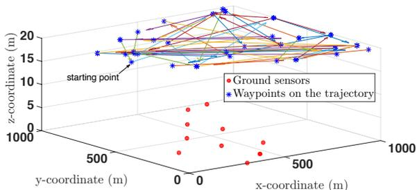
Fig. 6: Training the trajectory planning of the UAV given 50 waypoints.
