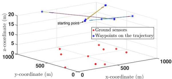
Fig. 5: Training the trajectory planning of the UAV given 10 waypoints.
