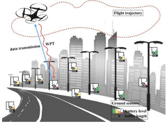
Fig. 1: Employing a UAV for aerial data collection and WPT, where wireless powered ground sensors are deployed for environmental monitoring in the smart city.
