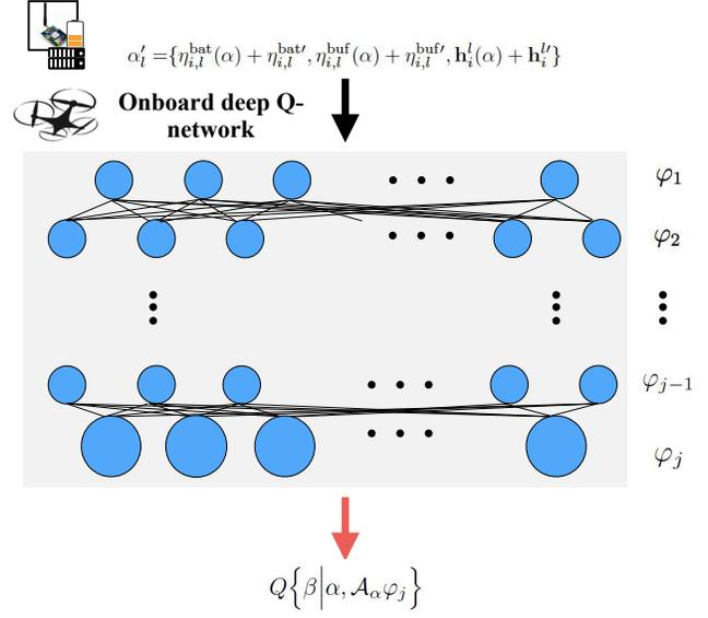
Fig. 3: The deep Q-network structure in DRLTP onboard the UAV.
