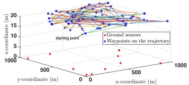
Fig. 7: Training the trajectory planning of the UAV given 80 waypoints.
