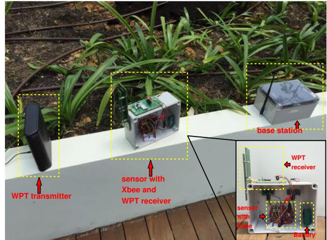
Fig. 3: The hardware setup contains the BS, WPT transmitter and sensor node with RFbee transceiver (for data transmission in 2.4 GHz) and WPT receiver.
