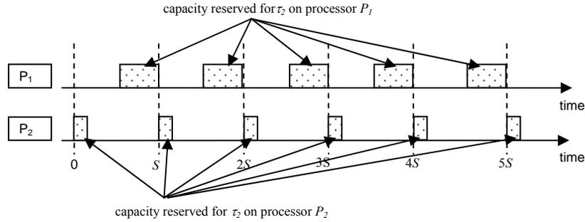
Figure 1. Slot-based split-task dispatching: How to perform run-time dispatching of a task that is assigned to two processors. A white rectangle with black dots indicates capacity reserved for task  $\tau_2$ .
