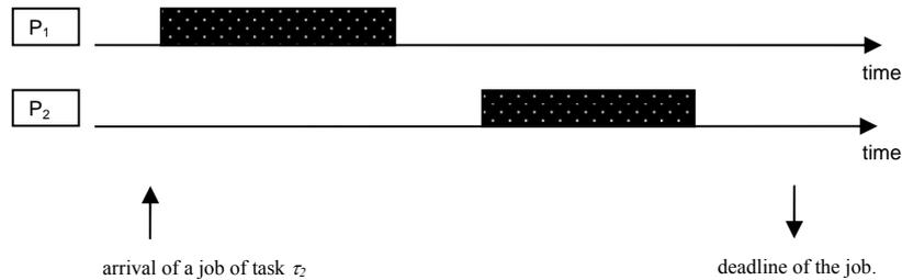
Figure 2. Job-based split-task dispatching: How to perform run-time dispatching of a task that is assigned to two processors. A dark rectangle with white dots indicates execution of the job of task  $\tau_2$ .
