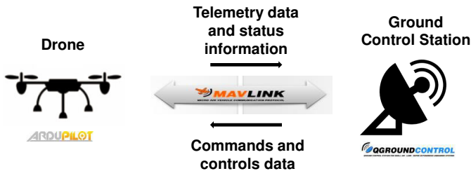
Fig. 1. Communication link between UAV and GCS.
