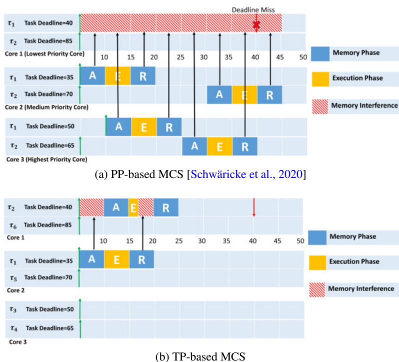
Figure 6.1: Inter-core memory interference
