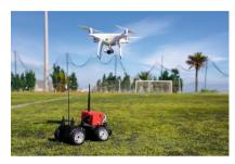
Fig 11: Prototype for the autonomous GPS tracking system, with the drone following a remote control vehicle.
