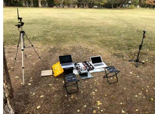
(b) Setup of the ground source node and the sink node.
