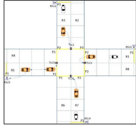
**Figure 1:** Grid-based Autonomous Intersection with MAS Communication.
