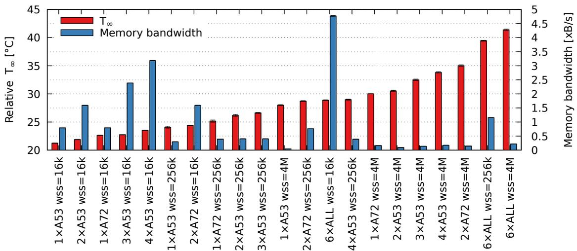
**Figure 14:** Memory performance and temperature (measured with the fan switched off)
