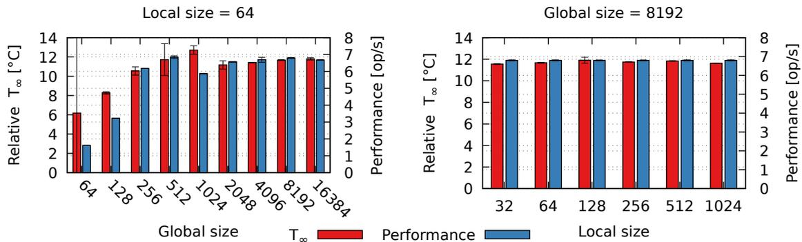
**Figure 11:** Performance of a compute-bound GPU benchmark
