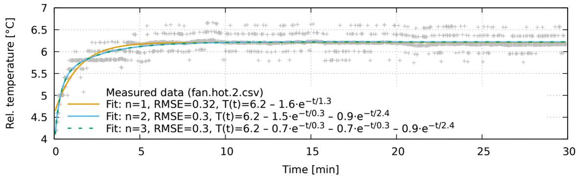
**Figure 7:** Measured data and fits with the fan switched on. Note that the ripples in the measured data are caused by compensation for ambient temperature.
