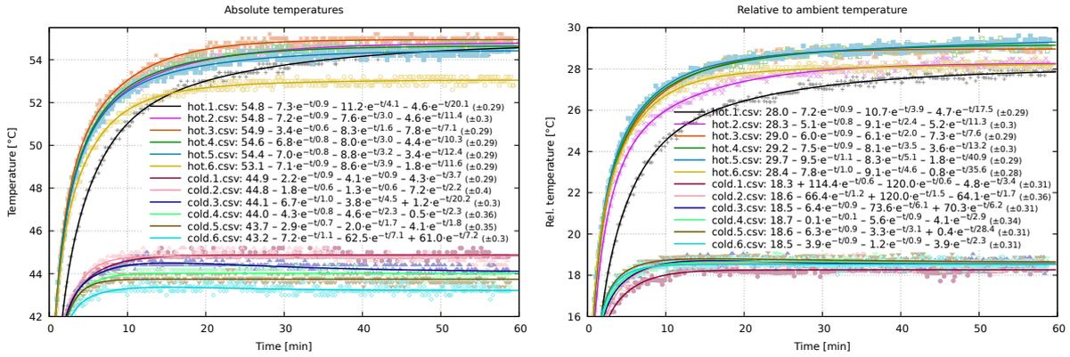
**Figure 5:** Comparison of model fitting with (right) and without (left) ambient temperature compensation. Fit error (RMSE) is given after  $\pm$  sign in parentheses.
