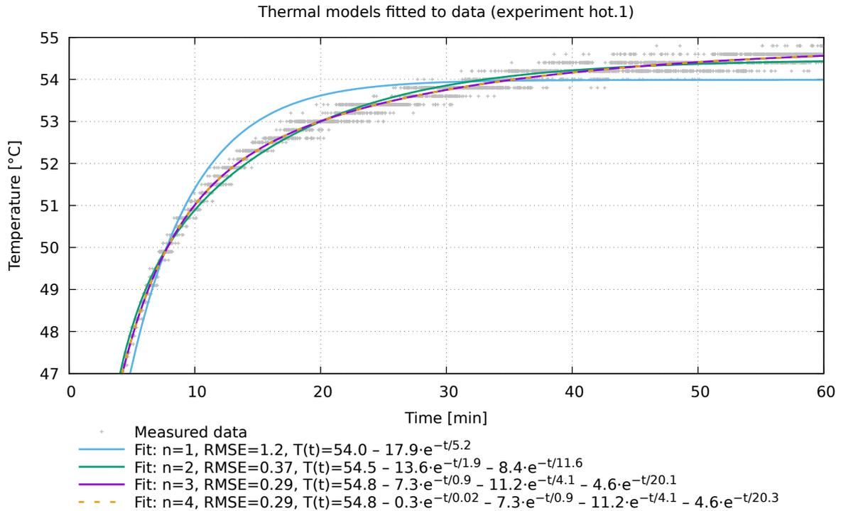
**Figure 3:** Measured data and fitted model (data < 47°C not visible)
