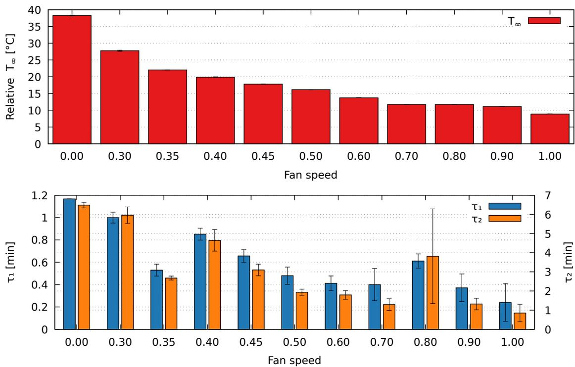
**Figure 9:** Relation between different fan speeds and estimated thermal model parameters. Note that 0.3 is the lowest speed that makes the fan move.
