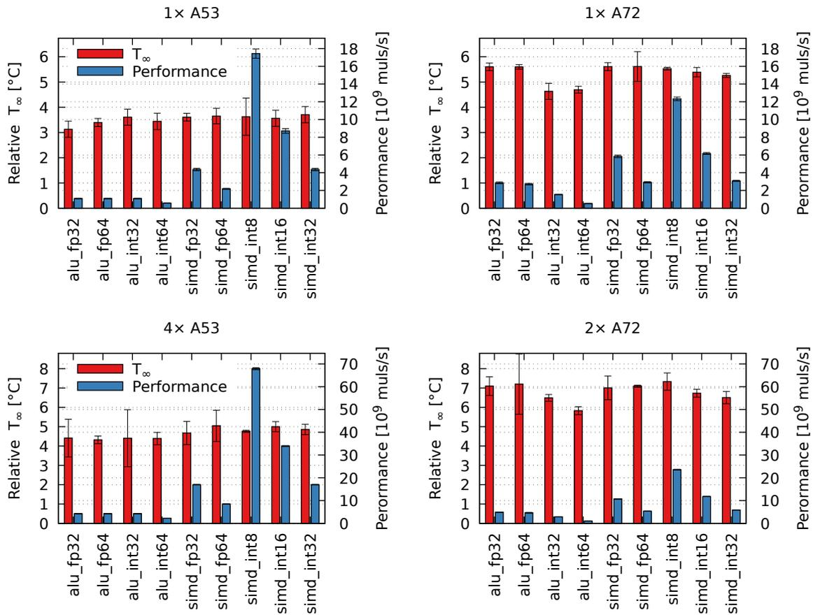
**Figure 10:** Comparison of relative steady state temperature  $T_{\infty}$  and performance of multiplication instructions on different CPUs.
