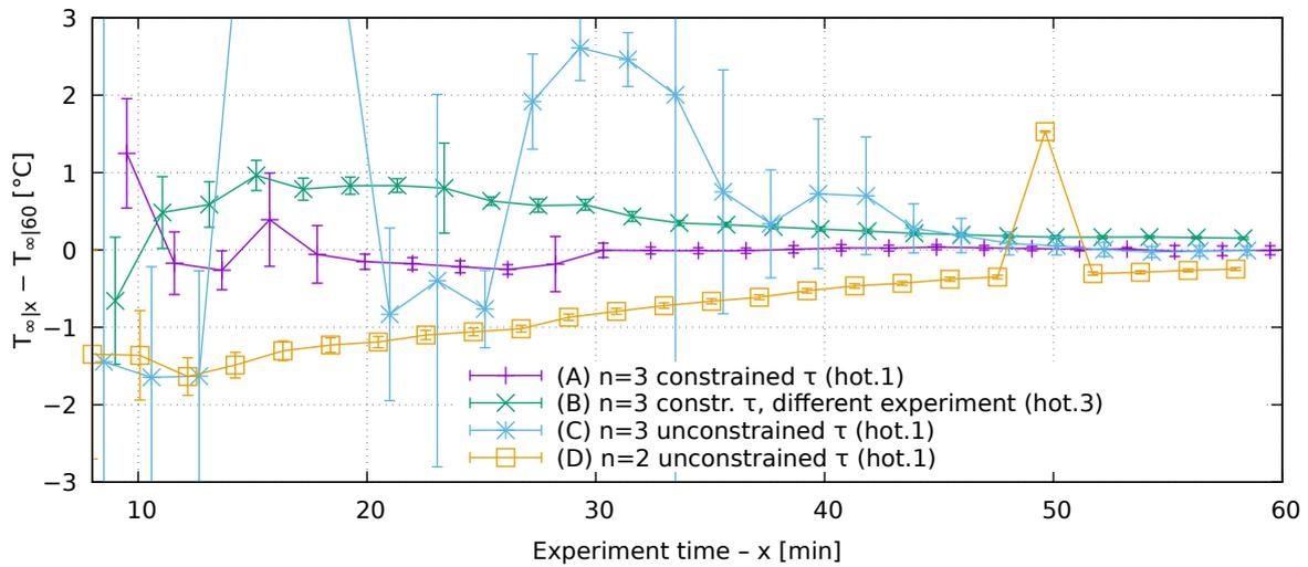
**Figure 6:** Relation between the length of the experiment and estimation of  $T_{\infty}$ . Vertical axis shows the difference between  $T_{\infty}$  estimated from data of length  $x$  ( $T_{\infty|x}$ ) and from full 60 minutes of data ( $T_{\infty|60}$ ). Error bars represent 95% confidence intervals.
