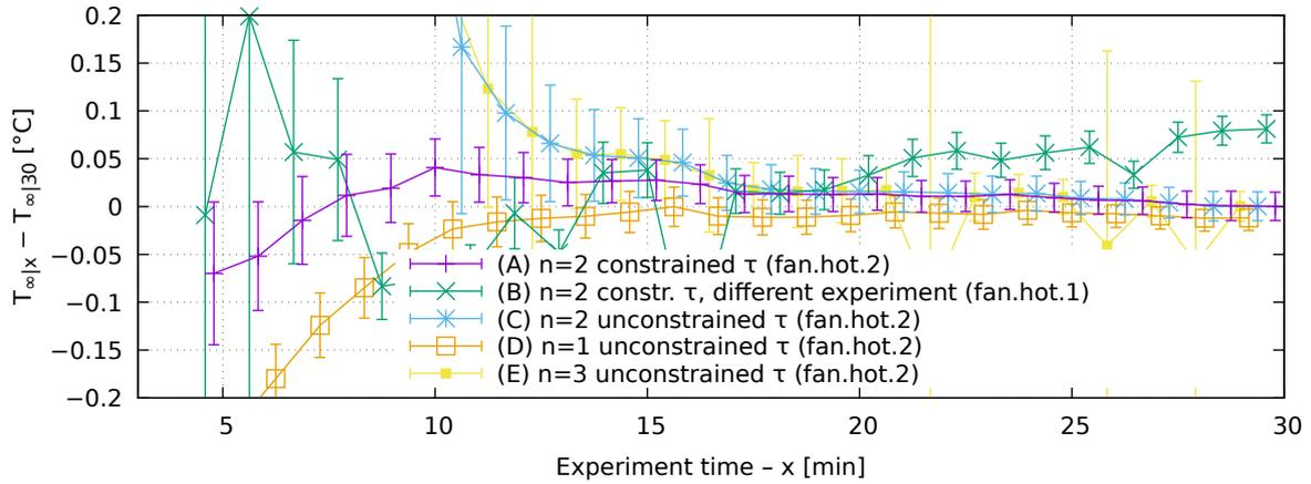
**Figure 8:** Relation between the length of the experiment and estimation of  $T_{\infty}$ . Vertical axis shows the difference between  $T_{\infty}$  estimated from data of length  $x$  ( $T_{\infty|x}$ ) and from full 30 minutes of data ( $T_{\infty|30}$ ). Error bars represent 95% confidence intervals.
