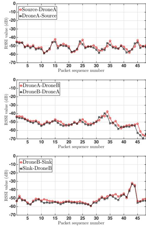
**Figure 2: RSS measurements of the airborne channels.**
