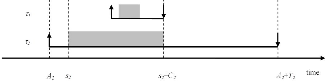
Fig. 1. All non-preemptive scheduling algorithms have the utilization bound 0.
