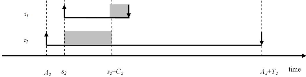
Fig. 2. An example that shows where a non-preemptive scheduling algorithm misses a deadline at a non-zero utilization.
