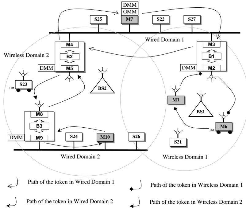
**Fig. 1.** Hybrid wired/wireless MLR PROFIBUS network example
