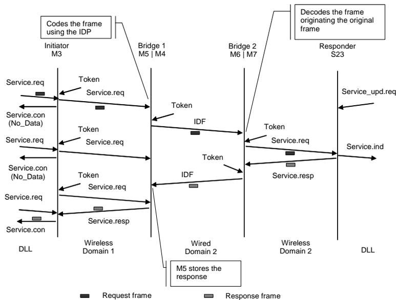
**Fig. 2.** Example for an Inter-Domain Transaction (IDT)
