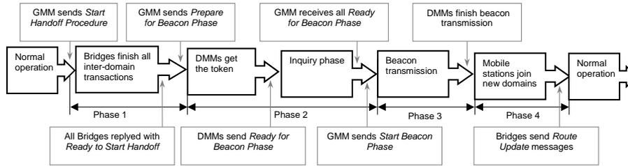
**Fig. 3.** Phases of the inter-cell mobility procedure
