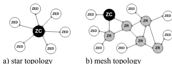
Fig 2. ZigBee star and mesh network topologies
